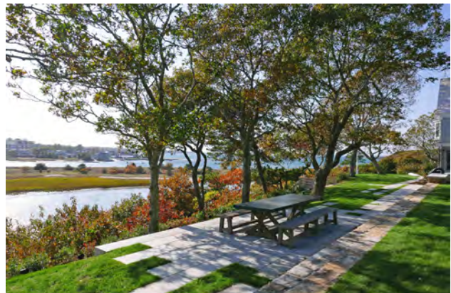
Figure 6-33. Example accessible picnic area: concrete or paver extension adjacent to walkway (TL Studio).
